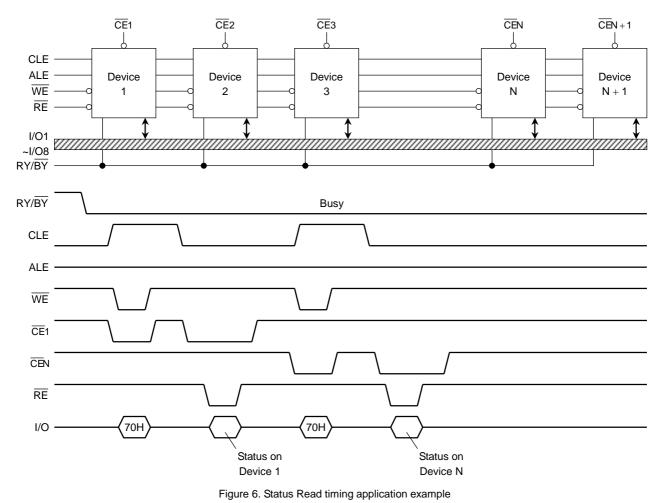
System Design Note: If the  $RY/\overline{BY}$  pin signals from multiple devices are wired together as shown in the diagram, the Status Read function can be used to determine the status of each individual device.
