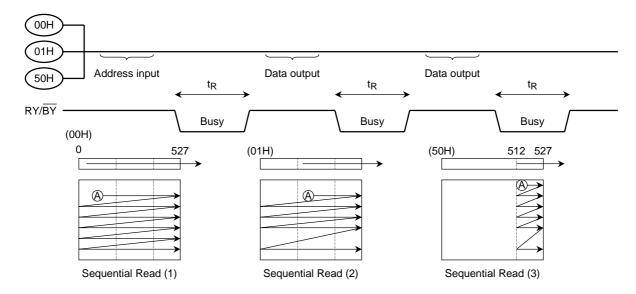
Sequential Read modes (1) and (2) output the contents of addresses  $0\sim527$  as shown above, while Sequential Read mode (3) outputs the contents of the redundant address locations only. When the pointer reaches the last address, the device continues to output the data from this address \*\* on each  $\overline{\text{RE}}$  clock signal.
