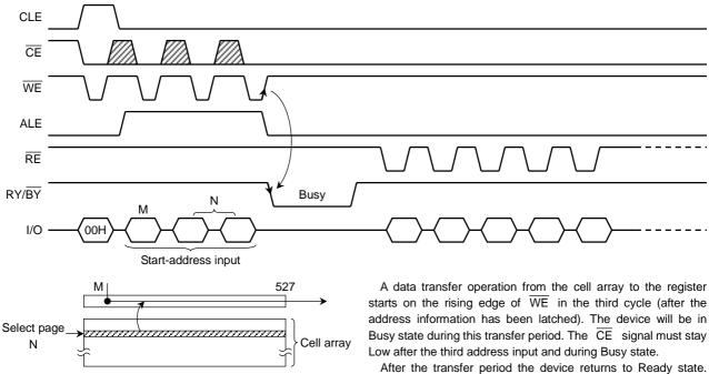
Figure 3. Read mode (1) operation
