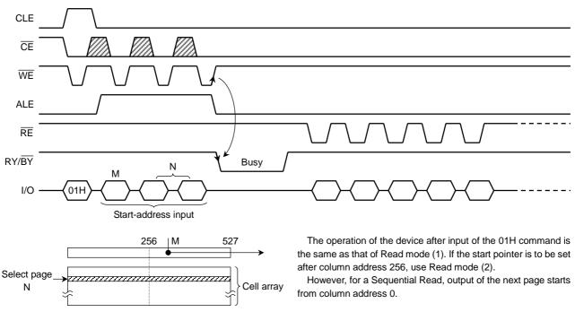
Figure 4. Read mode (2) operation
